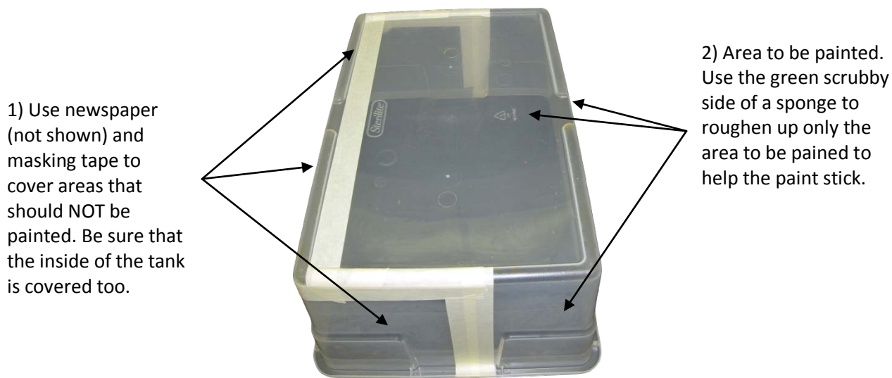
Figure 1. Storage box with masking tape borders to use as a guide for painted versus not painted areas. Arrows indicate areas that should be painted white and areas that should be masked off during painting and remain clear. A picture of a painted water tank is included in the MATERIALS PHOTO GUIDE – Lesson 1: Water Stratification (Teacher Supplies) .
